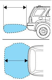
While receiving a warning the radio volume will be reduced to a predetermined level. After the warning goes away, the radio will return to the previous value. The RSS automatically turns on when the gearshift lever is placed in R (Reverse) and the ignition is on. A control in the message center allows the driver to disable the system, refer to Message center in the Instrument Cluster chapter for more information.
